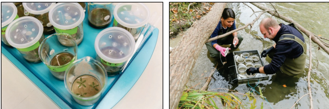
Figure 20: Sediment toxicity test with the aquatic plant Myriophyllum aquaticum (left) and sediment sampling in the Venoge river, Lausanne (right).
