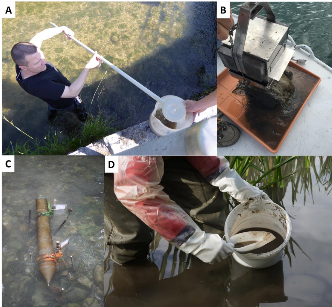
Figure 5: Different sampling devices that can be used in the field. A) Telescopic sampler B) Ekman grab sampler C) Time-integrated suspended tube sampler D) Scoop.
