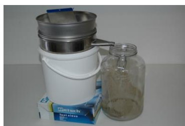
Figure 8: Sieving system to isolate the fraction <63 \mu\text{m} (Photo: canton Bern).
