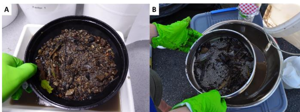
Figure 7: Example of wet sieving at 2 mm. (A) Off site with inert equipment for trace metal analysis and (B) In situ with inert equipment for organic micropollutant analysis.
